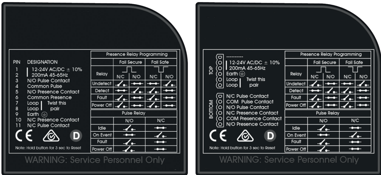
Figure 9. Example of LC20-1 side labels. Power supply requirements and pin connections are clearly stated on the side of the unit. 11 Pin configuration is shown on the left and DIN Rail version on the right
